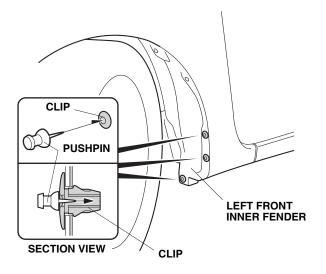
2. Using a pushpin, pierce the center of the three clips on the left front inner fender.
