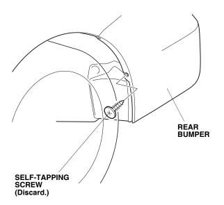
6. Secure the left rear splash guard using two 5 x 25 mm self-tapping screws tightened in the order shown.
